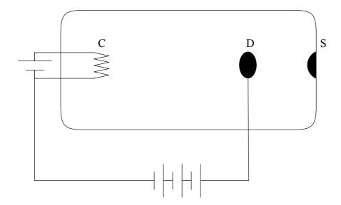
The cathode rays were formed at C and were accelerated toward the solid disc at D. A clear shadow of the disc is formed at S. A bar magnet held near the tube between C and D caused the shadow to move.
